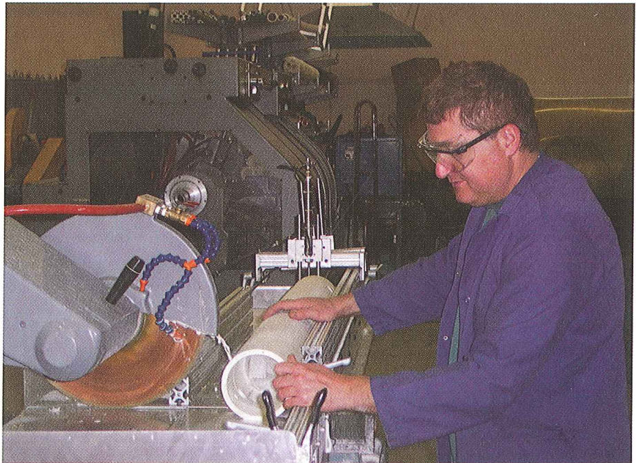
Skilled ceramic machinist Joao (John) Demai works 50+ hours a week cutting, drilling, grinding, and milling ceramic and quartz pieces to very high tolerances. Here he is cutting a 4½-in. diameter dense mullite tube to length.
